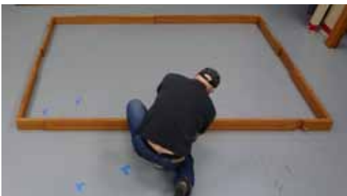
Setting up the bath; note: the wooden frame is adjustable, allowing size to be custom fit for each object.
